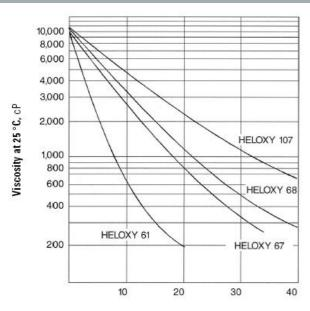
Weight percent of Epoxy Functional Modifier in Blends with EPON™ Resin 828
